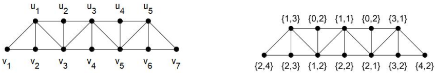
(a) Warren with verticals truss graph modelled (b) Warren with verticals truss graph with multiset representation of each vertex
